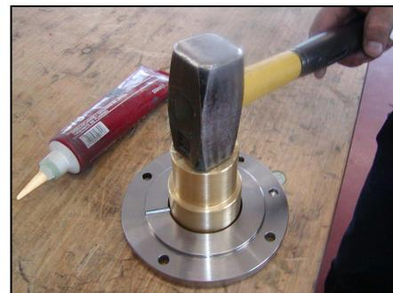
*Insert until stop the oil seal, using a insertion punch and a hammer.*
