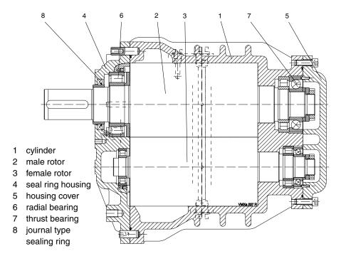
**Performance data:** intake pressure  $p_1 = 1$  bar, intake temperature  $t_1 = 20$  °C
